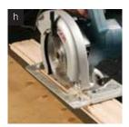
Remove the lower edge of the groove on the end and side of the board.
